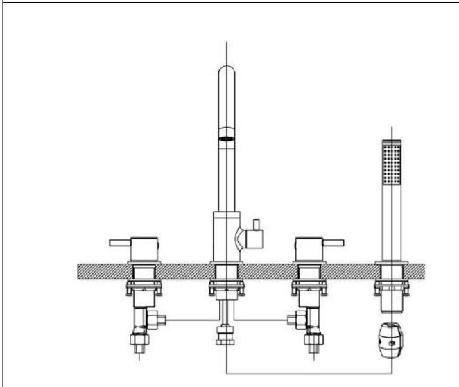
Connect the hot valve and cold valve with the isolation valves(not included) by connecting hoses, hot on the left, cold on the right.
