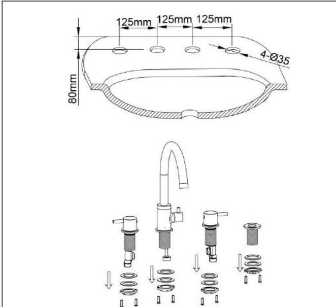
Remove the Screws, Locknuts, Metal Gaskets, and Rubber Gaskets from the Legs of each body.
